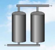
**Iron Sponge Treatment** - Iron sponge treatment is another biogas treatment process that removes hydrogen sulfide from biogas. The process design and costing uses input parameters such as the bed height, superficial gas velocity, reactor contact time, media properties (e.g., bulk density, iron sponge grade, number of cycles, regeneration time, regeneration efficiency) and cost metrics (\$/Ib of Iron sponge, \$/ft2 of vessel).
